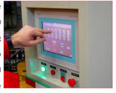
operation the operator can check the load and the stroke of each cylinder. The Cylinder Accuracy is ± 3%. Jacking Layer under Climbing Jack Frame (CJF) made by steel blocks is easily handled by operator / riggers (with a maximum weight of 20 kg for each steel).
